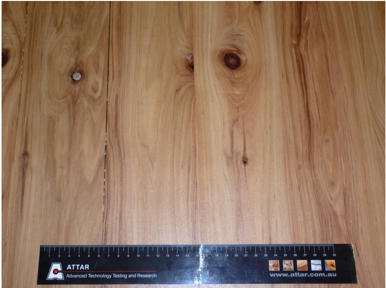
Figure 1: Timber board applied with One coat AQUAPRO 8020 sealer. One coat AQUAPRO 8068 with AQUAPRO 8930 Sure Grip Additive. One coat AQUAPRO 8068.
