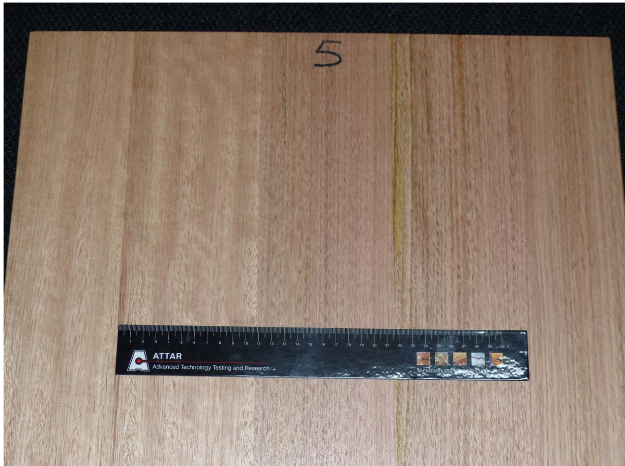
Figure 1: One coat FASTASEAL 3030 Clear Sealer. One coat DURAPOL 1045 SUPER GLOSS. One coat DURAPOL 1014 LOW SHEEN containing Polycure 3920 High Grip applied to timber board.
