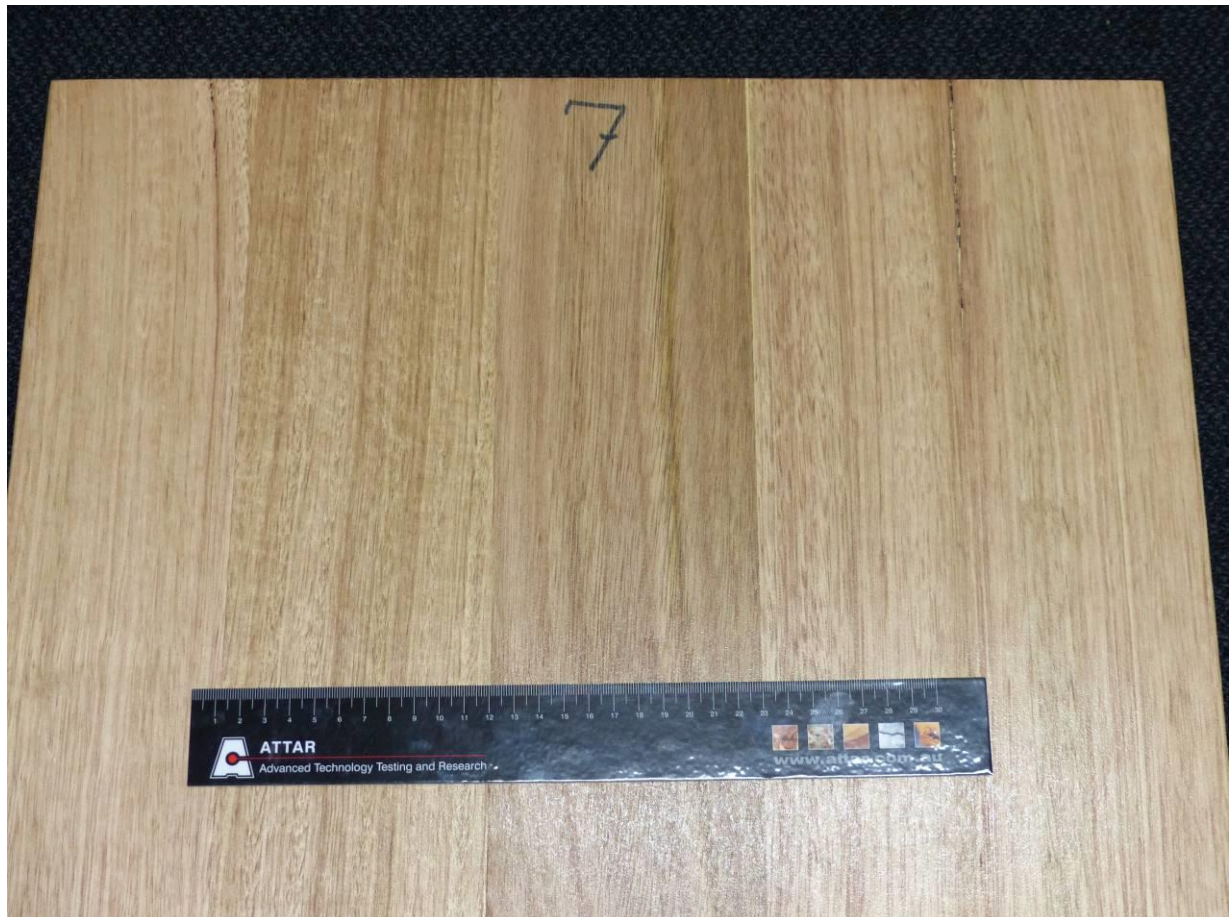
Figure 1: One coat FASTASEAL 3030 Clear Sealer. One coat NATUROIL 3100 Oil Modified Gloss. One coat NATUROIL 3100 Oil Modified Gloss containing Polycure 3920 High Grip applied to timber board.
