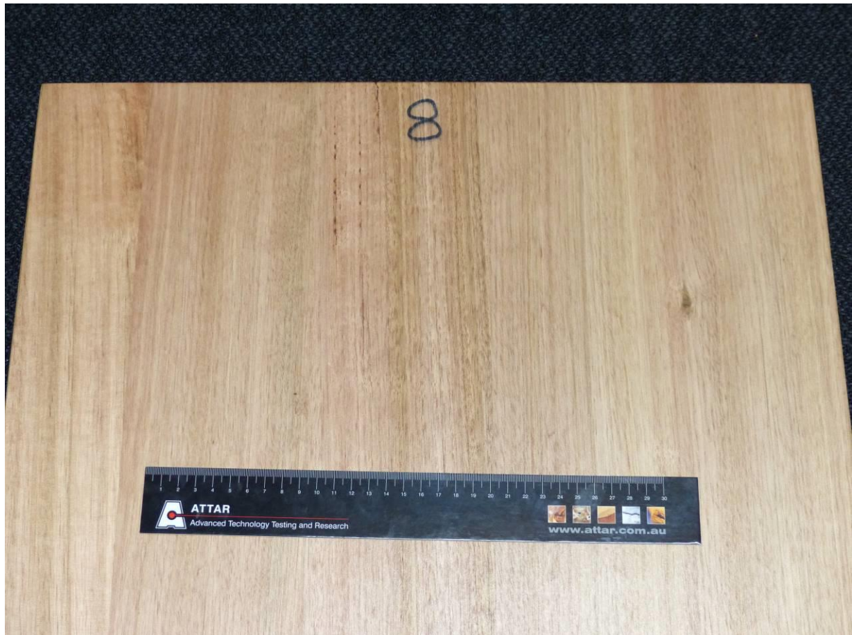
Figure 1: One coat FASTASEAL 3030 Clear Sealer. One coat NATUROIL 3100 Oil Modified Gloss. One coat NATUROIL 3115 Oil Modified Low Sheen containing Polycure 3920 High Grip applied to timber board.
