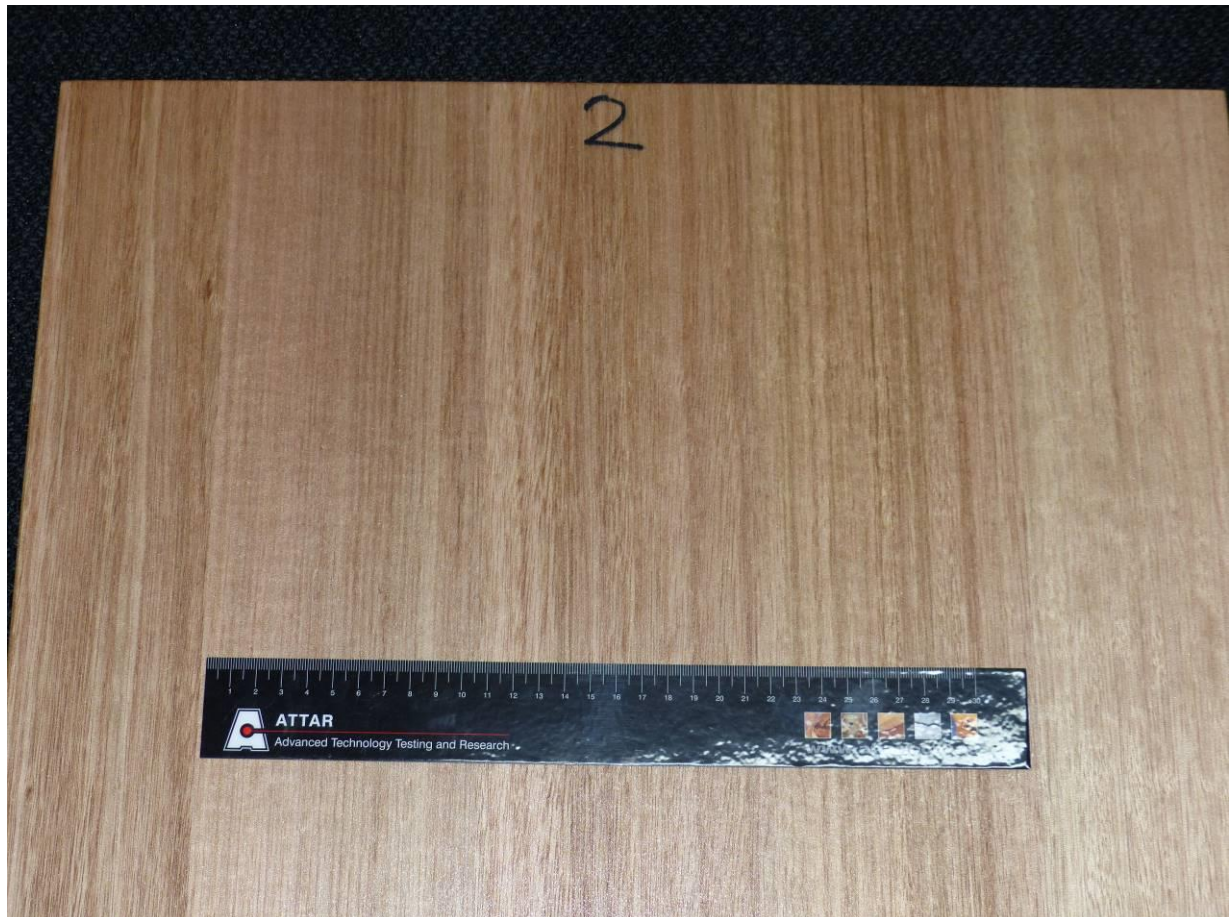
Figure 1: One coat FASTASEAL 3030 Clear Sealer. One coat TITAN GLOSS. One coat TITAN GLOSS containing Polycure 3920 High Grip applied to timber board.
