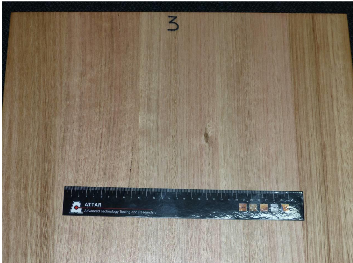
Figure 1: One coat FASTASEAL 3030 Clear Sealer. One coat DURAPOL 1045 SUPER GLOSS. One coat DURAPOL 1012 SEMI GLOSS containing Polycure 3920 High Grip applied to timber board.
