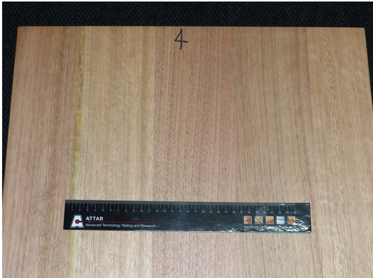
Figure 1: One coat FASTASEAL 3030 Clear Sealer. One coat DURAPOL 1045 SUPER GLOSS. One coat DURAPOL 1013 SUPER SATIN containing Polycure 3920 High Grip applied to timber board.
