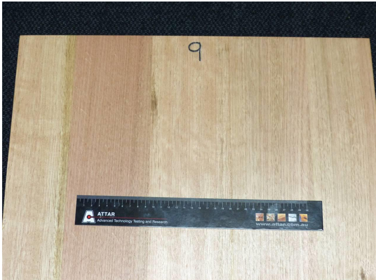
Figure 1: One coat FASTASEAL 3030 Clear Sealer. One coat NATUROIL 3120 TUNG OIL Low Sheen Sealer. One coat NATUROIL 3120 TUNG OIL Low Sheen Sealer containing Polycure 3920 High Grip applied to timber board.
