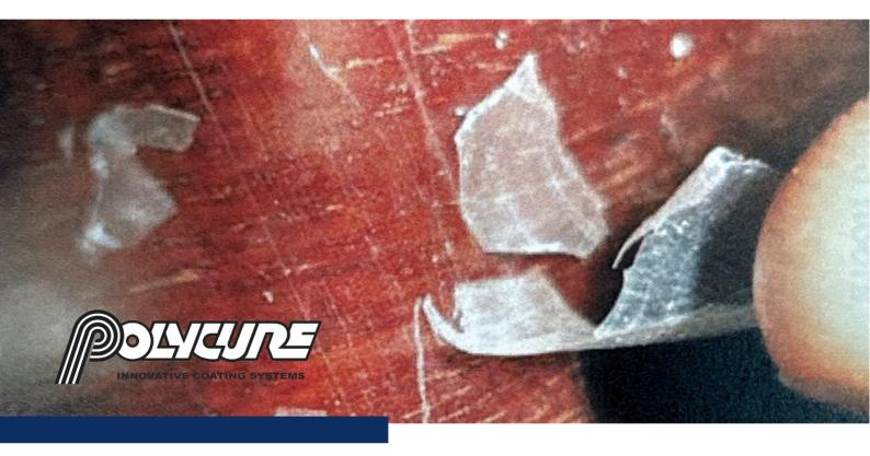
Delamination is the failure to adhere it may be:
