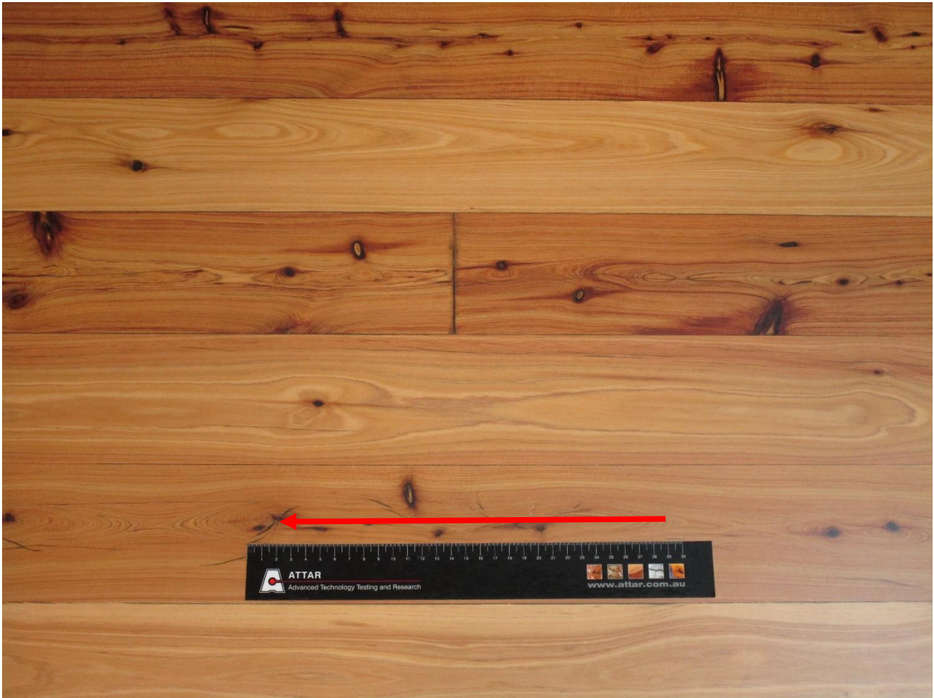
Figure 1: DURAPOL Silky Matt. 3 Coat System. 1 x Coat FASTSEAL 3030 Clear Sealer, 2 x Coat DURAPOL Silky Matt. Arrow indicates direction of test.
