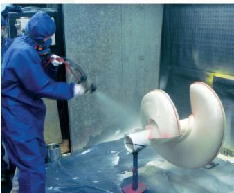
applications where elastomeric coatings/linings are specified. They also remain flexible so are capable of handling the expansion and contraction of metal associated with climate change and the movement or cracking in concrete.
